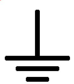
or with "G," "GR," "GRD," "Ground," "Grounding," or other equivalent marking.
