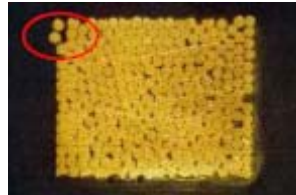
Figure 4.3.5.a Example cross sectional view of an unacceptable weld bond due to strands not in contact with the weld bond.
