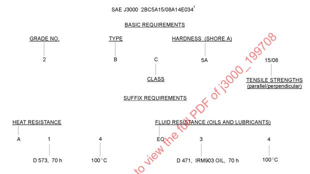
In this example, the basic requirements for heat aging resistance and resistance to volume change resulting from oil immersion are superseded by suffix requirements.
