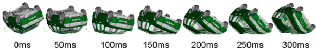
FIGURE 37 - SIMULATION OF ROOF-TO-GROUND PORTION OF ROLLOVER EVENT USING LS-DYNA
