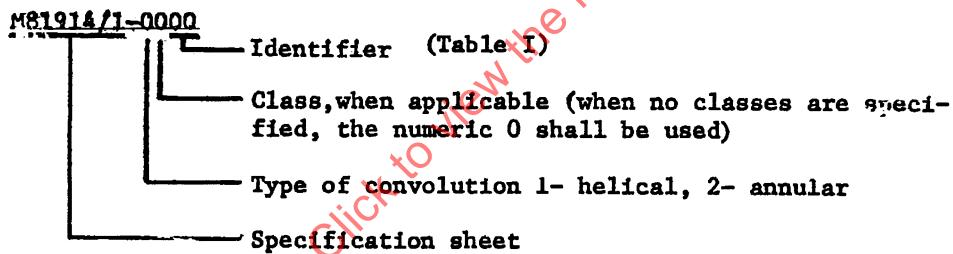
Standard convolution Polytetrafluoroethylene, standard wall, 0.500 inch is identified as: M81914/1-1106.
