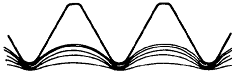
FIGURE 2 PLAN LINES ROLLED THREAD
