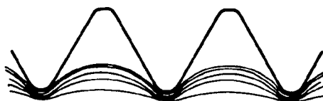
FIGURE 2 FLOW LINES ROLLED THREAD
