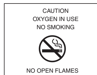
FIGURE A.9.6.3.2 A Suggested Minimum Text for Precautionary Signs.
