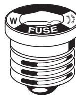
FIGURE 8.6.2.1.1(a) A Typical, Edison-Based Nonrenewable Fuse, Single Element, for Replacement Purposes Only.
