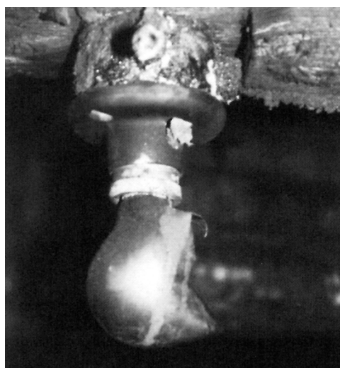
FIGURE 6.2.15 A Typical “Pulled” Bulb Showing That the Heating Was from the Right Side.
