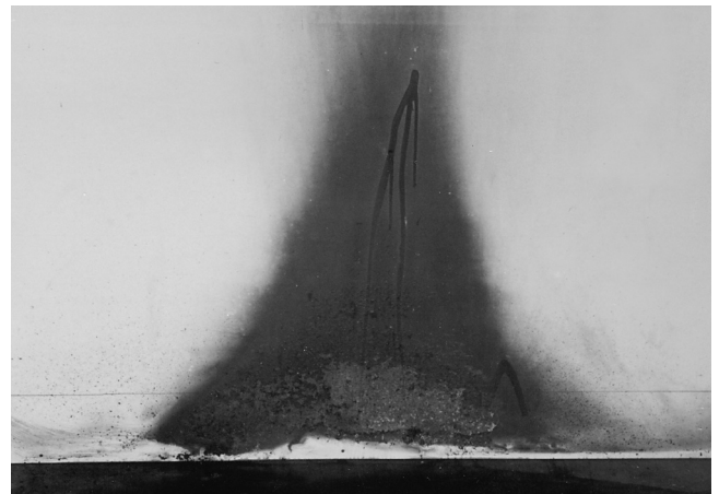
FIGURE 6.3.7.2(b) Inverted Cone Pattern Produced by Burning a Small Pile of Newspapers.
