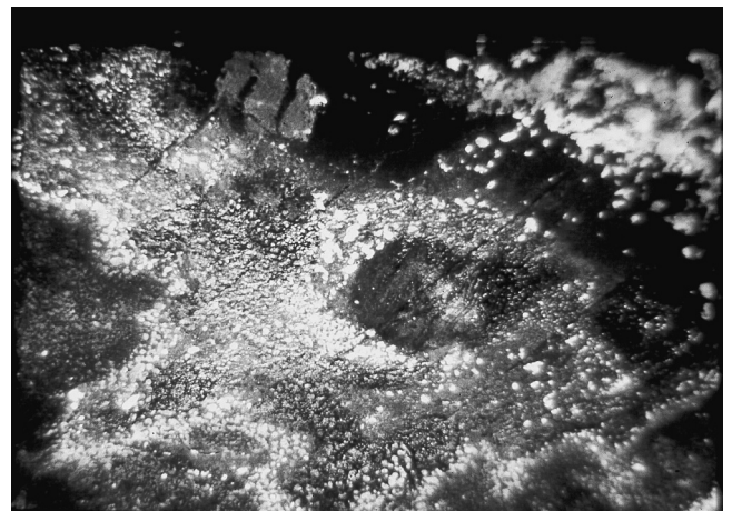
FIGURE 6.3.7.9(a) Doughnut-Shaped Fire Pattern on a Carpeted Floor.
