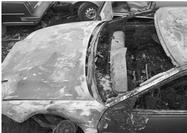
FIGURE 25.8.1.2(b) Radial Pattern on the Driver's Side Door Produced by an Engine Compartment Fire.
