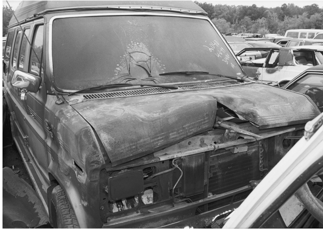
FIGURE 25.8.1.2(a) Incipient Windshield Failure Caused by an Engine Compartment Fire.
