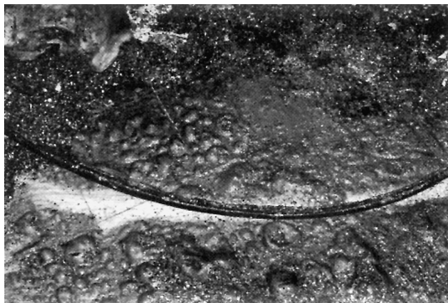
FIGURE 15.2.6.6.3 Floor Tile Protected from Radiant Heat by Wire.
