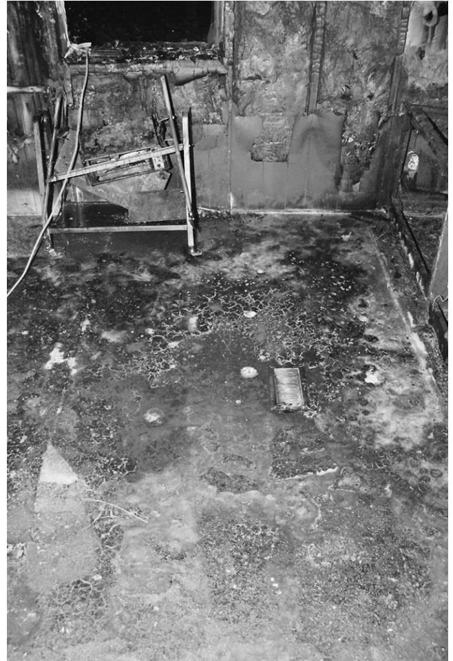
FIGURE 6.3.7.8.5(b) Fire Patterns on Linoleum Floor Resulting from Fully Developed (Post-Flashover) Fire in Full-Scale Test Burn of Residential Structure; No Ignitable Liquids Were Present.
