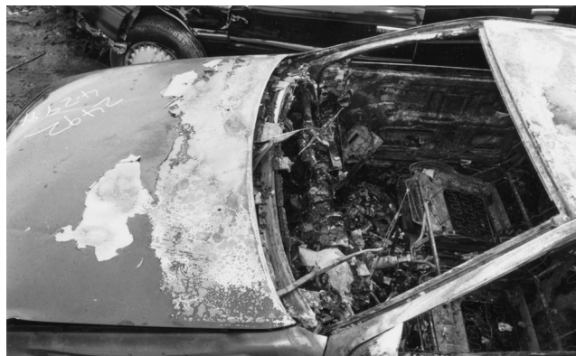
FIGURE 25.8.1.1(c) Radial Fire Pattern Produced by a Passenger Compartment Fire.
