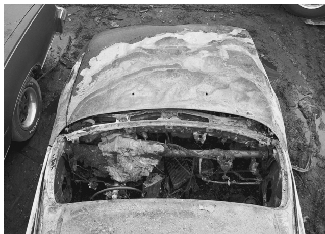
FIGURE 25.8.1.1(d) Another Radial Fire Pattern Produced by a Passenger Compartment Fire.
