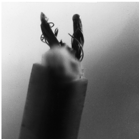
FIGURE 8.10.3.1(c) Stranded Copper Conductors Severed by Arcing through Charred Insulation with the Strands Terminated in Beads.
