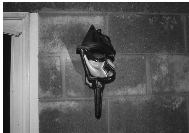
FIGURE 6.2.8.4 Melted Plastic Lighting Fixture, Indicating Heating from Right to Left.
