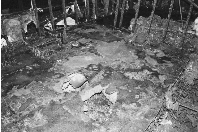
FIGURE 6.3.7.8.5(a) Fire Patterns on Floor Resulting from Fully Developed (Post-Flashover) Fire in Full Scale Test Burn of Residential Structure. Floor Was Carpeted and Room Had Typical Residential Furnishings; No Ignitable Liquids Were Present.
