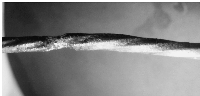
FIGURE 8.10.6.2.1(a) Stranded Copper Conductor in Which Melting by Fire Caused the Strands to Be Fused Together.
