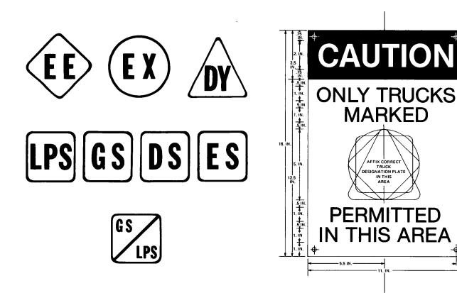
Figure 5-4.2.2. Markers to identify type of industrial truck. The markers for LPS, GS, DS, ES, and GS/LPS are 4 in. (102 mm) square. The width of the others is 5 in. (127 mm). The signs shall have black borders and lettering on a yellow background.
