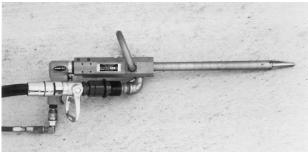
FIGURE 11.4.4 Skin Penetrator Agent Applicator Tool (SPAAT).
