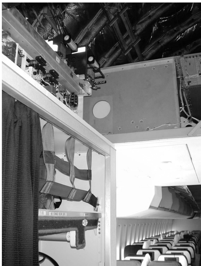
FIGURE 13.5(b) Location of Flight Data Recorder and Cockpit Voice Recorder.
