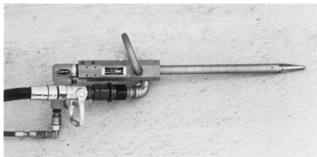
FIGURE 11.4.4 Skin Penetrator Agent Applicator Tool (SPAAT).
