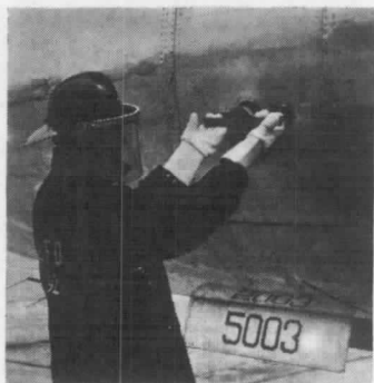
Figure A-23C. Normal entry at main entry door — first pull door handle outward.
