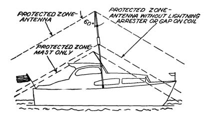
Diagrams above illustrate the "cone of protection" provided by a grounded mast or antenna. This protective zone is largely immune to direct strokes of lightning. No part of the vessel to be protected should extend outside the cone of protection. Thus in the cabin cruiser illustrated, adequate lightning protection is afforded only by the grounded antenna equipped with a lightning arrester or gap on the coil.
