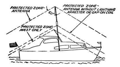
Diagrams above illustrate the "cone of protection" provided by a grounded mast or antenna. This protective zone is largely immune to direct strokes of lightning. No part of the vessel to be protected should extend outside the cone of protection. Thus in the cabin cruiser illustrated, adequate lightning protection is afforded only by the grounded antenna equipped with a lightning arrester or gap on the coil.
