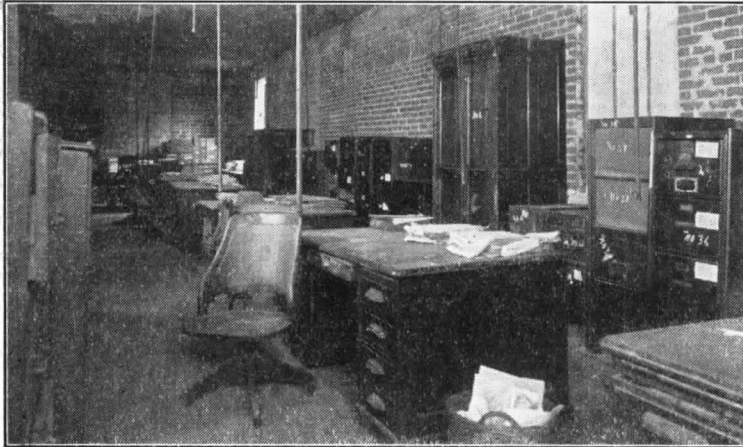
Fig. 3—Test room representing office with 20 lbs. per sq. ft. combustible contents. Wood finish floor, wood furniture.
