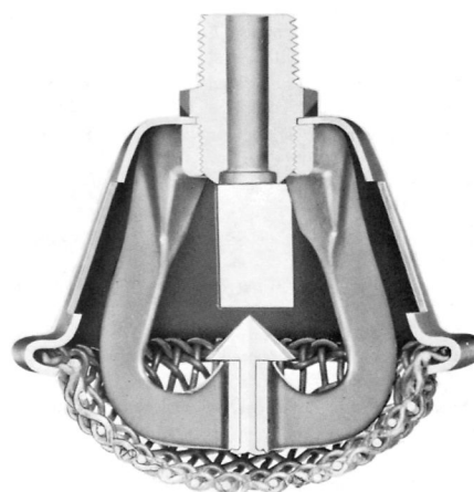
FIGURE A.3.3.6.4 Foam-Water Spray Nozzle.
