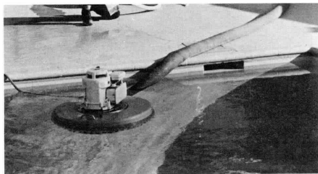
Figure E-1-2.6 Floating 500-gpm pump in swimming pool supplying the department pumper through large diameter hose.
