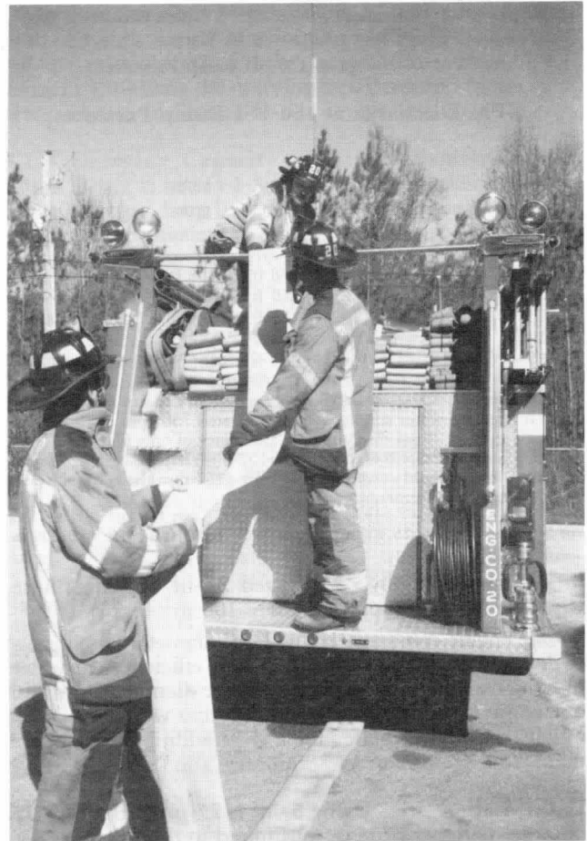
Figure D-1-6(d) Fire fighters quickly reload 5-in. hose as the driver straddles the hose. Note that the hose is loaded over the bar between the stanchions.
