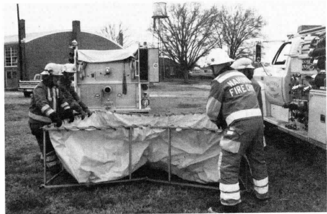
Figure C-1-13(a) Portable drop tanks should be simple to set up. Note the portable tank compartment (door open) on the tanker. (Photo by Nahunta Volunteer Fire Department, North Carolina)
