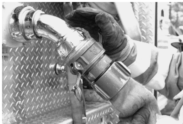
FIGURE C.11 Example of a Quick Connect Coupling That Can Help to Reduce the Fill Time.
