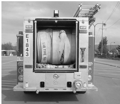
FIGURE D.4 Apparatus with Reels for Large-Diameter Hose. (Courtesy of LLNL Fire Department)
