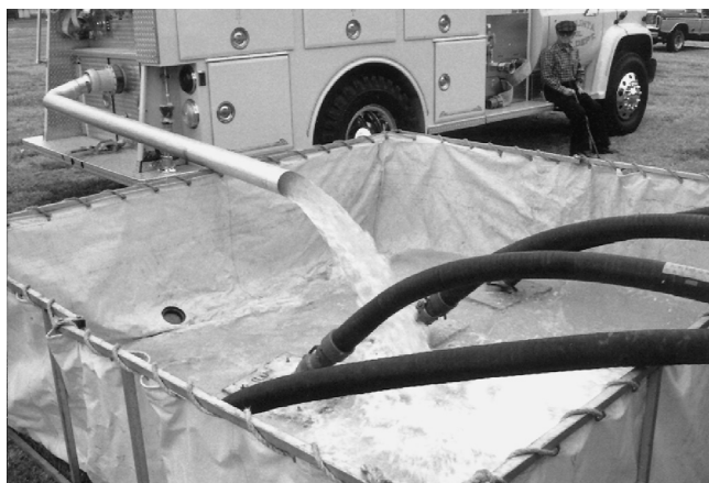
FIGURE C.15 Portable Drop Tank with “L”-Shaped Aluminum Irrigation Discharge Pipe.
