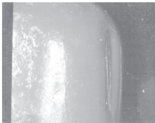
Figure A.4 — Dent containing cut or gouge
