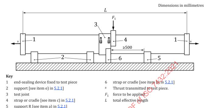
Figure 2 — Test arrangement for tests detailed in 9.3 and 9.4
