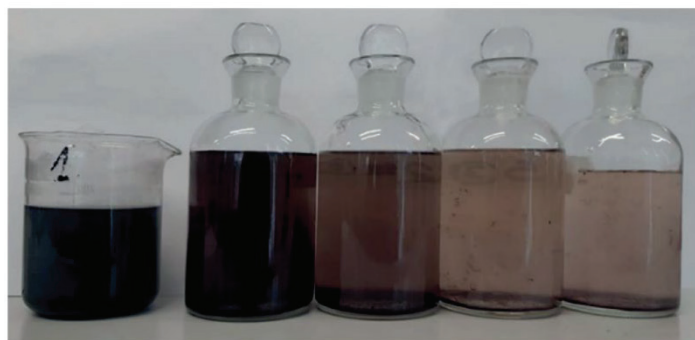
Figure 3 — Water samples treated with different hydrogen peroxide volume fractions of 15 %
