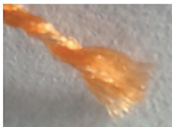
Figure 6 — Example of polyamide thread with 180 filaments
