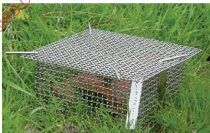
Figure F.2 — “Open” microcosms, covered by netting maintained by pickets [1]
