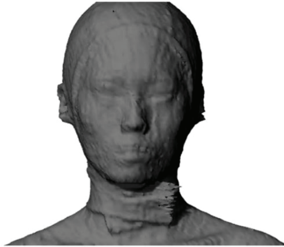
Figure 4 — An inappropriate scan result with significant noise
