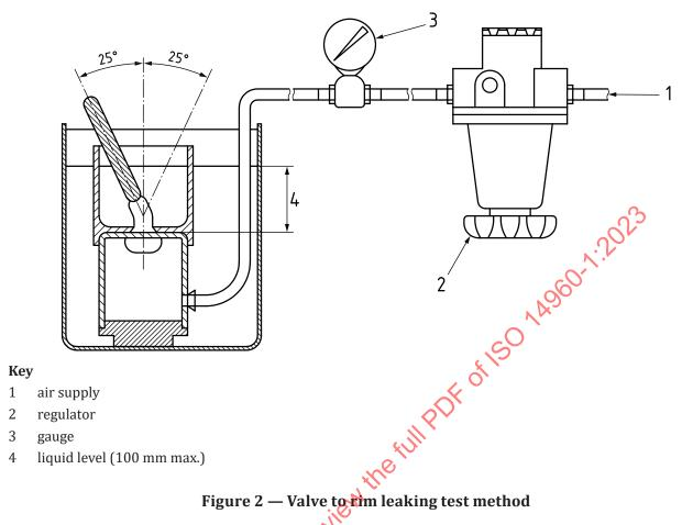
Figure 2 — Valve to rim leaking test method
