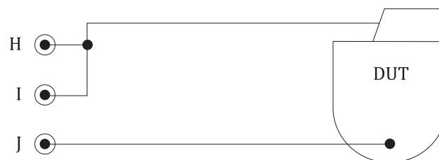
Figure 14 — Connection to a single-channel unipolar device
