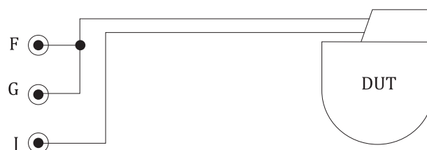
Figure 6 — Differential mode connection to single-channel bipolar device
