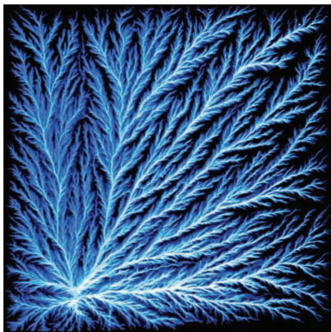
Figure 10: An electrostatic discharge caused by electron accumulation in an insulator: such discharges are a major cause of anomalies on satellites and have proved difficult to suppress © K A Ryden
