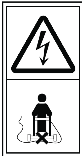
Figure AA.4 – Product safety label illustrating – "WARNING – Keep the supply cord away from the tines"
