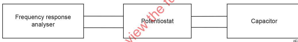
Figure B.1 – Capacitance measurement system by the low frequency AC method
