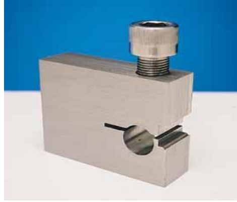
Figure 2 - Bolt-Loaded Compact Specimen
