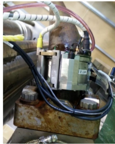
Figure 10-26: Transducer for both 2 and 21/2 NPS sized manipulators. The transducer fires tangentially to the inspection surface with the sound redirected via a mirror.
