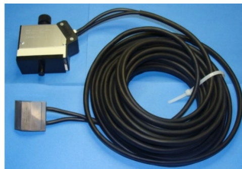
Figure 10-26: Transducer for both 2 and 21/2 NPS sized manipulators. The transducer fires tangentially to the inspection surface with the sound redirected via a mirror.
